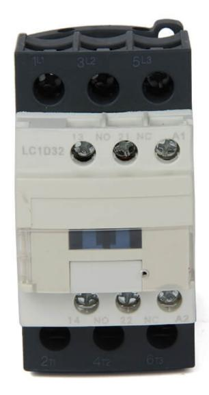
CJX2-DN series AC Contactors are suitable for frequency 50/60Hz, rated insulation voltage up to 1000V, rated operation current 9-150A under AC-3 duty. It is mainly used for making and breaking electric circuits at a long distance & for frequent starting, stopping & controlling AC Motors. It is used in combination with thermal relay to compose a magnetic motor starter. The products comply with IEC60947-4.
