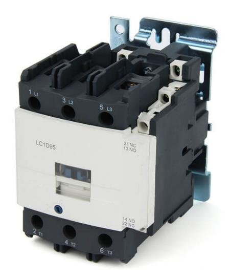
CJX2-DN series AC Contactors are suitable for frequency 50/60Hz, rated insulation voltage up to 1000V, rated operation current 9-150A under AC-3 duty. It is mainly used for making and breaking electric circuits at a long distance & for frequent starting, stopping & controlling AC Motors. It is used in combination with thermal relay to compose a magnetic motor starter. The products comply with IEC60947-4.
